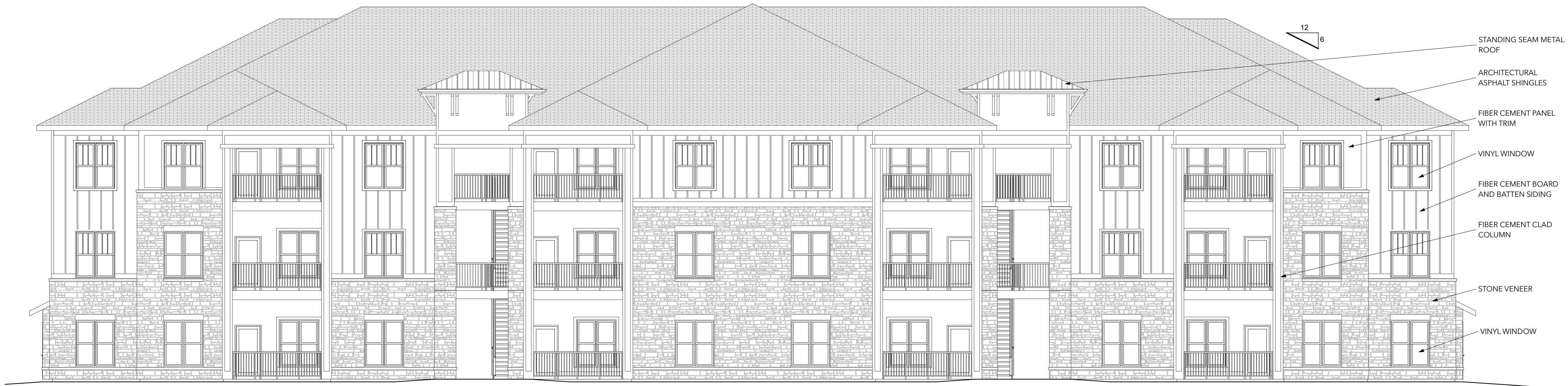
3 BUILDING TYPE 4 FRONT ELEVATION SCALE: 1/8" = 1'-0" SIDING: 44% GLAZING: 25% MASONRY: 31%
