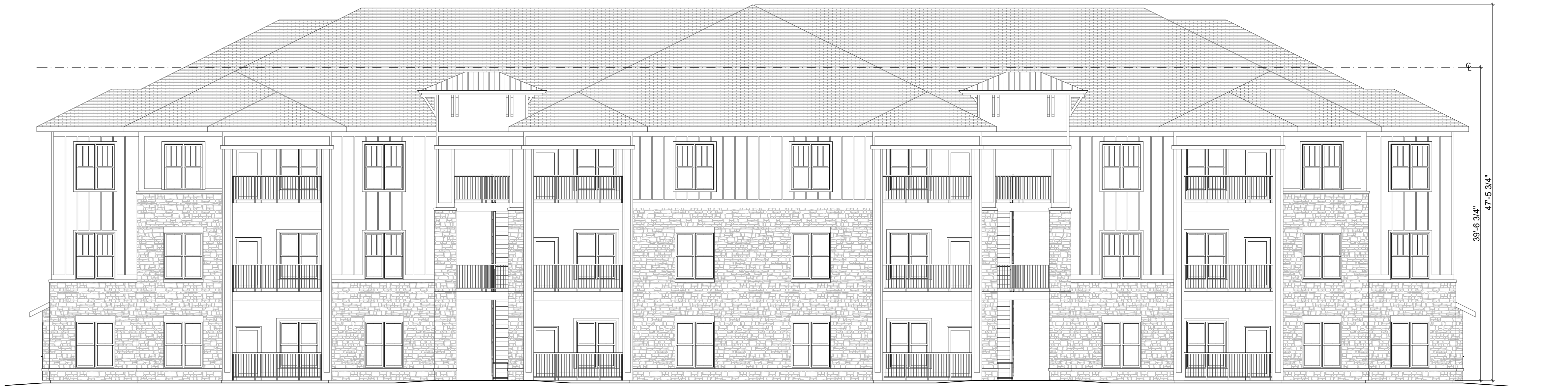
4 BUILDING TYPE 4 REAR ELEVATION SCALE: 1/8" = 1'-0" SIDING: 44% GLAZING: 25% MASONRY: 31%
